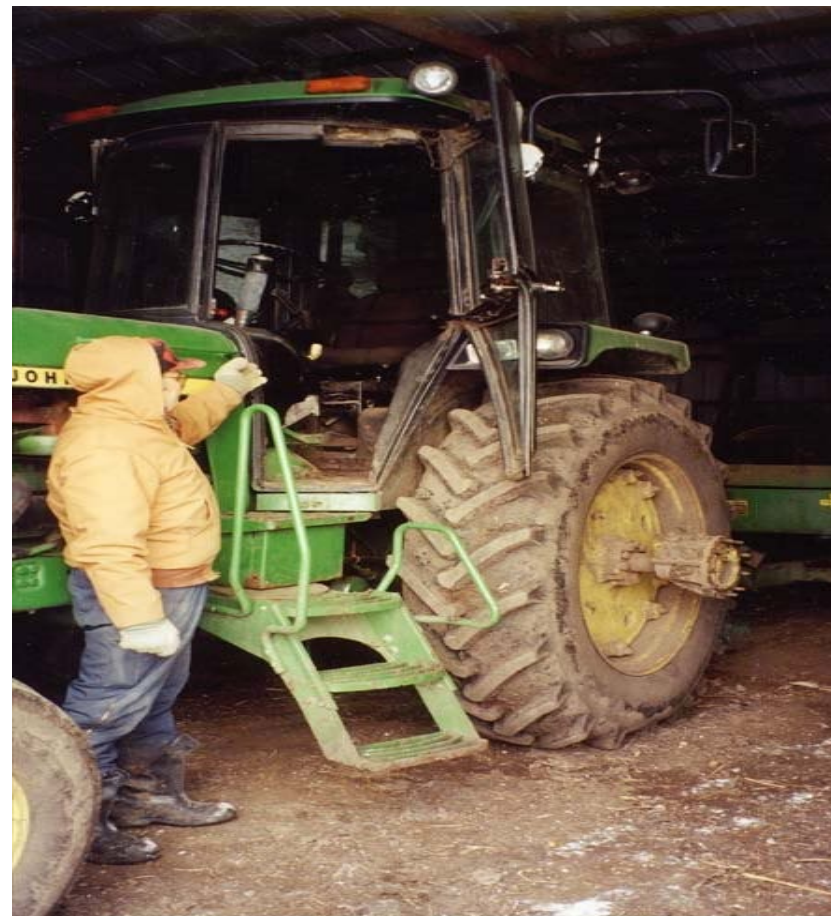
Modifications-Stair Extenders and Handrails
